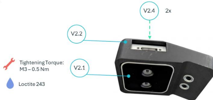
Figure 18: D405 Camera to Wrist Camera Mount
