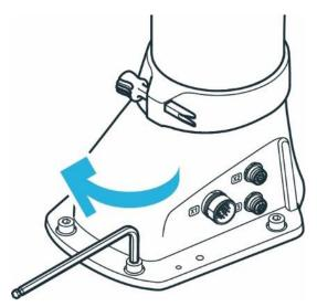
Figure 46: Mounting of the Arm
