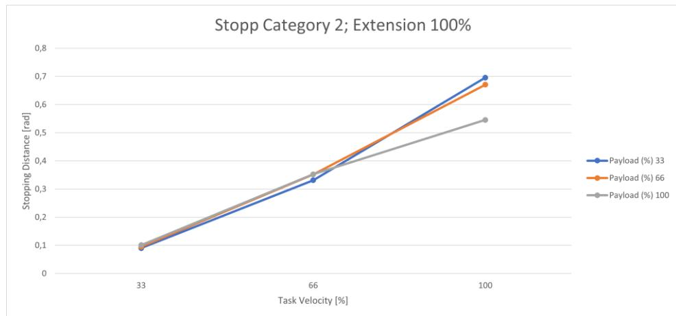
Fig. 17.40: Distance; Stopp Cat 2; Joint 3 100%
