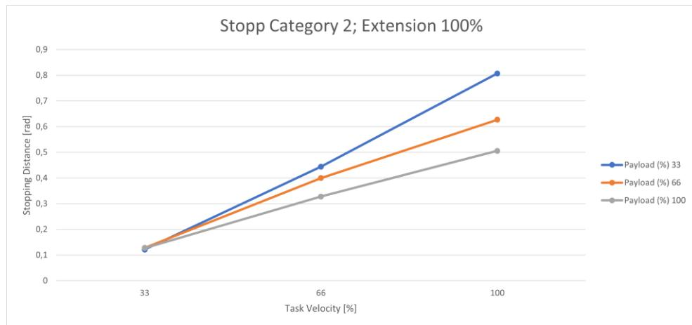
Fig. 17.28: Distance; Stopp Cat 2; Joint 1 100%
