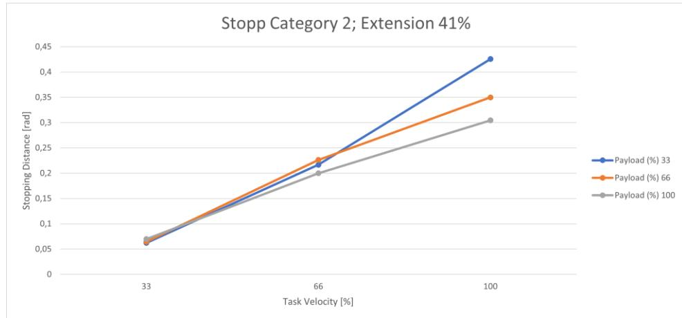
Fig. 17.36: Distance; Stopp Cat 2; Joint 3 41%
