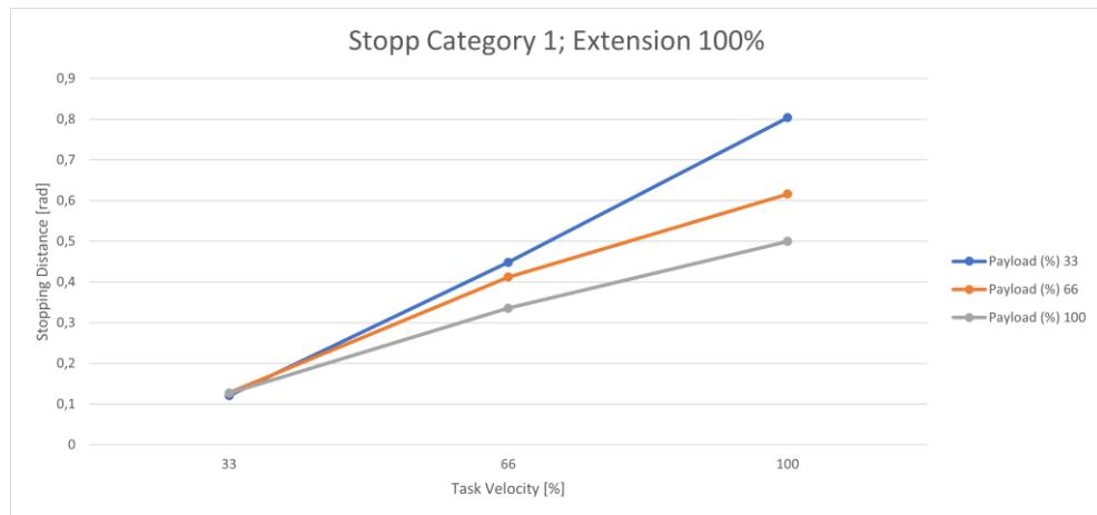
Fig. 17.6: Distance; Stopp Cat 1; Joint 1 100%
