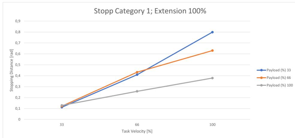
Fig. 17.12: Distance; Stopp Cat 1; Joint 2 100%
