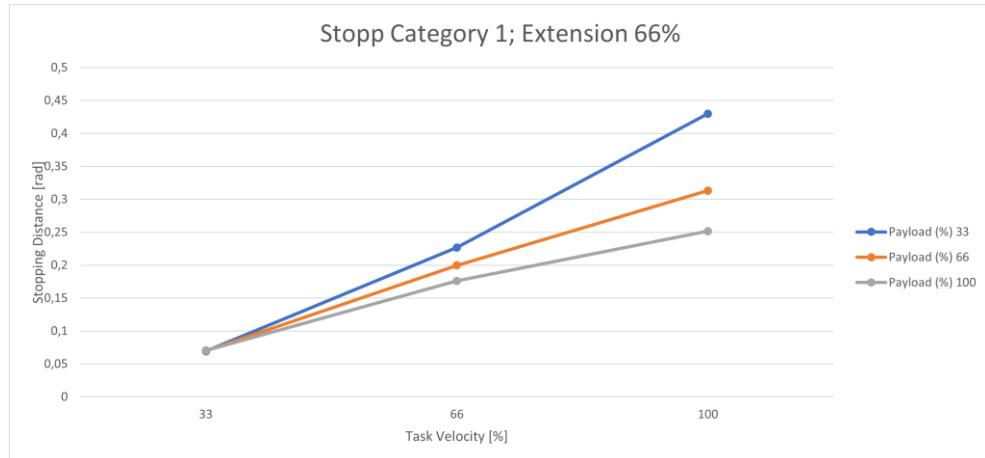
Fig. 17.20: Distance; Stopp Cat 1; Joint 4 66%
