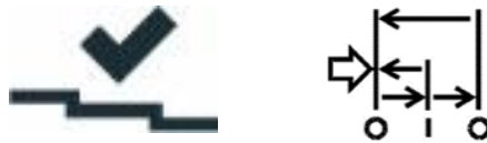
Fig. 6.4: switching status Enabling Button
