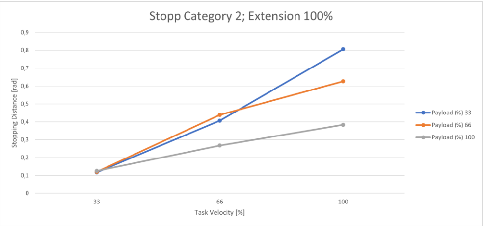
Fig. 14.34: Distance; Stopp Cat 2; Joint 2 100%
