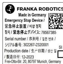
Fig. 3.8: Type label emergency stop device
