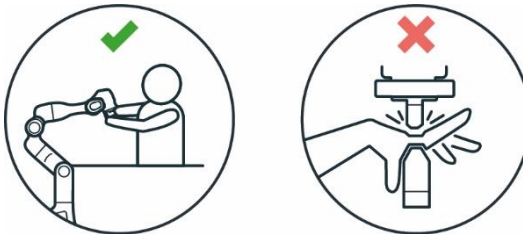
Fig. 7.31: Distance to arm Squeezing the hand
