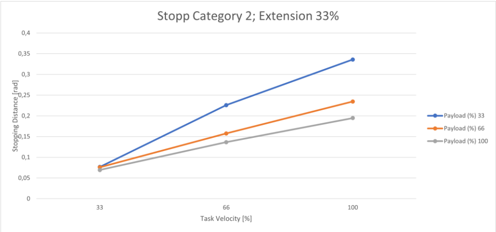
Fig. 14.30: Distance; Stopp Cat 2; Joint 2 33%
