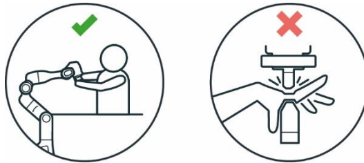
Figure 61: Distance to Arm squeezing the hand
