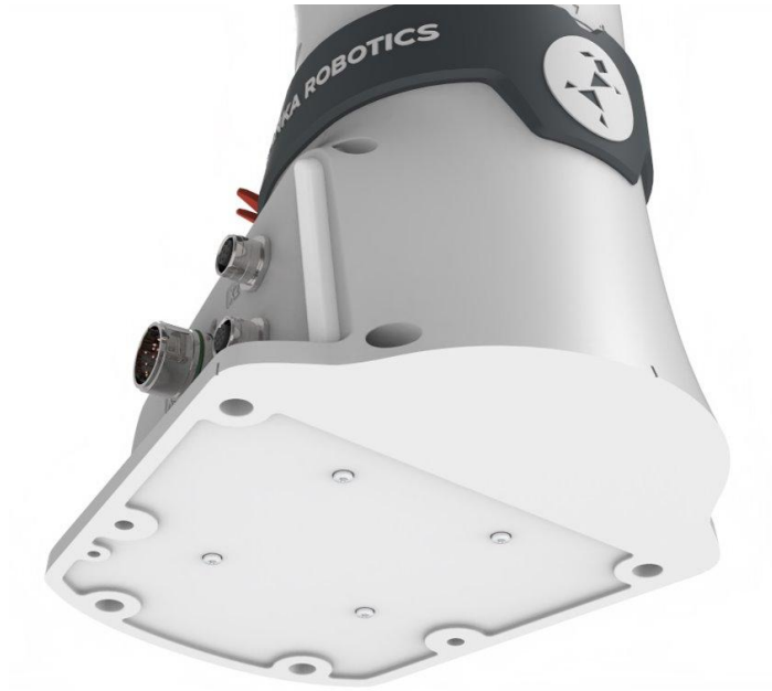
Figure 15: Base Alignment Marks
