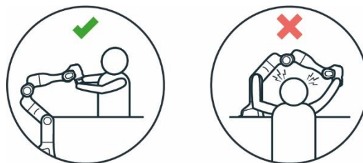
Figure 59: Distance to Arm bumping the head
