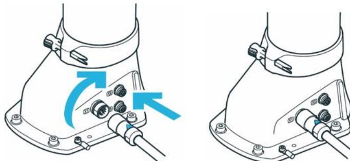
Figure 50: Connection of connecting cable to the Arm
