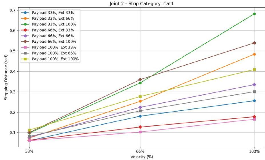
Figure 74: Distance, Stopp Cat1, Joint 2
