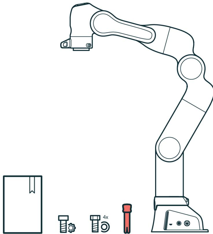
Figure 27: Scope of delivery Arm
