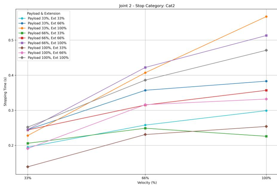
Figure 81: Time, Stop Cat2, Joint 2
