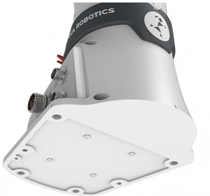
Figure 15: Base Alignment Marks
