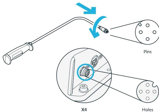
Figure 52: Connection of external Enabling Device
