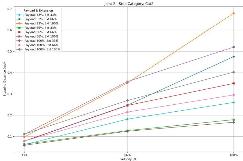
Figure 80: Distance, Stop Cat2, Joint 2
