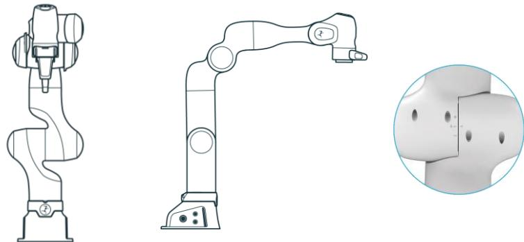
Figure 57: Joint reference position of the Arm
