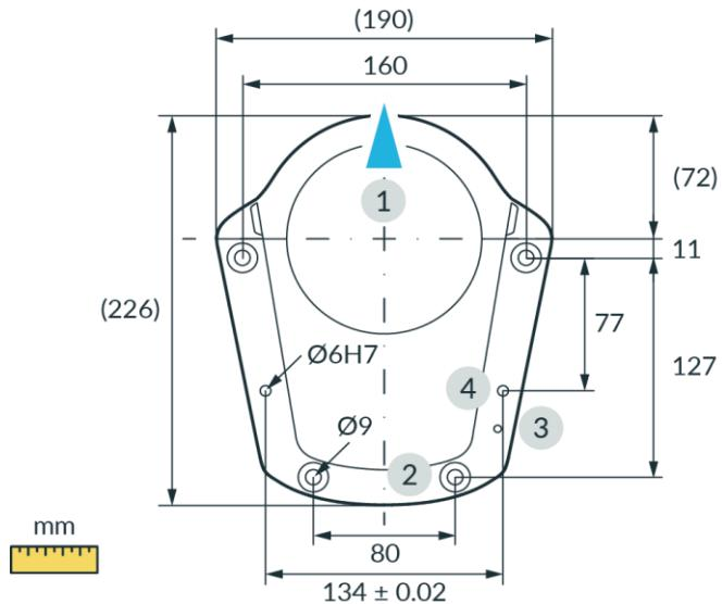
Figure 44: Drilling template
