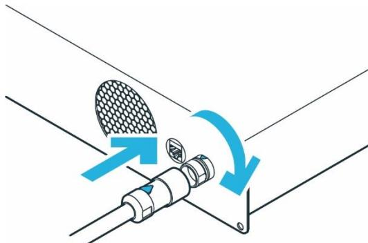
Figure 51: Connection of connecting cable to the control
