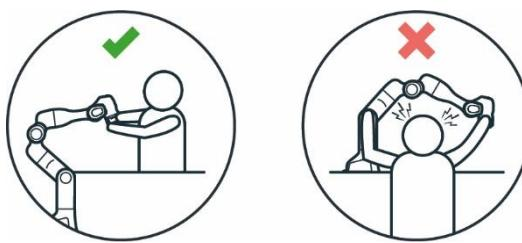
Figure 59: Distance to Arm bumping the head
