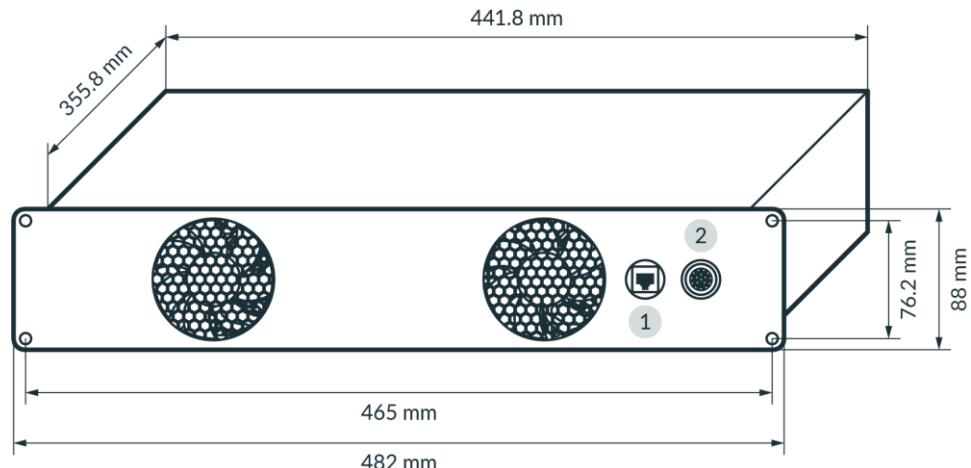
Figure 25: Dimensions and connection ports of control
